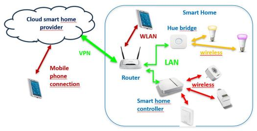
Communication between Smart Home Components and mobile devices. Drawing: M. Sorger
